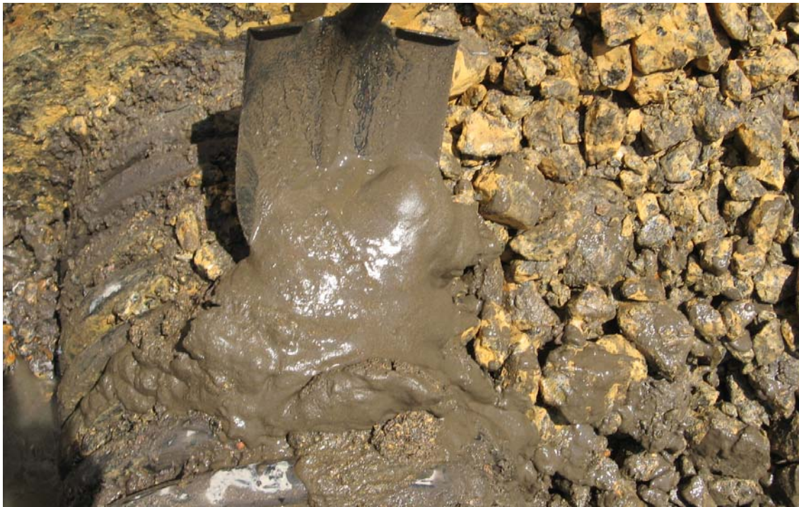
Photo 22. Solids washed from limestone in the Mitchell Tank.
