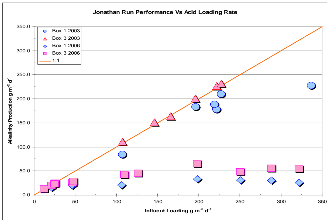
Figure B. Alkalinity generation rates at varying influent acidity loading rates for the Jonathan Run units.
