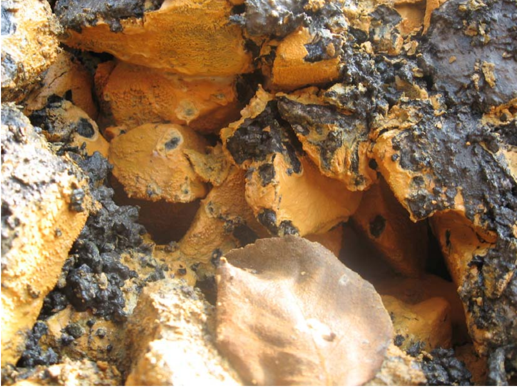
Photo 32. Open void spaces in scale coated limestone of the Mitchell Tank system.
