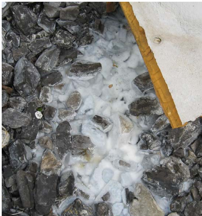
Photo 31. Suspended solids filling aggregate void spaces in the Jonathan Run Box 3 system.
