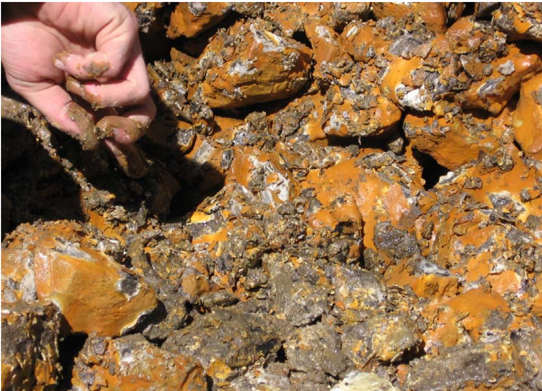
Photo 30. Scale flaking off of limestone in the Jonathan Run Box 1 system.
