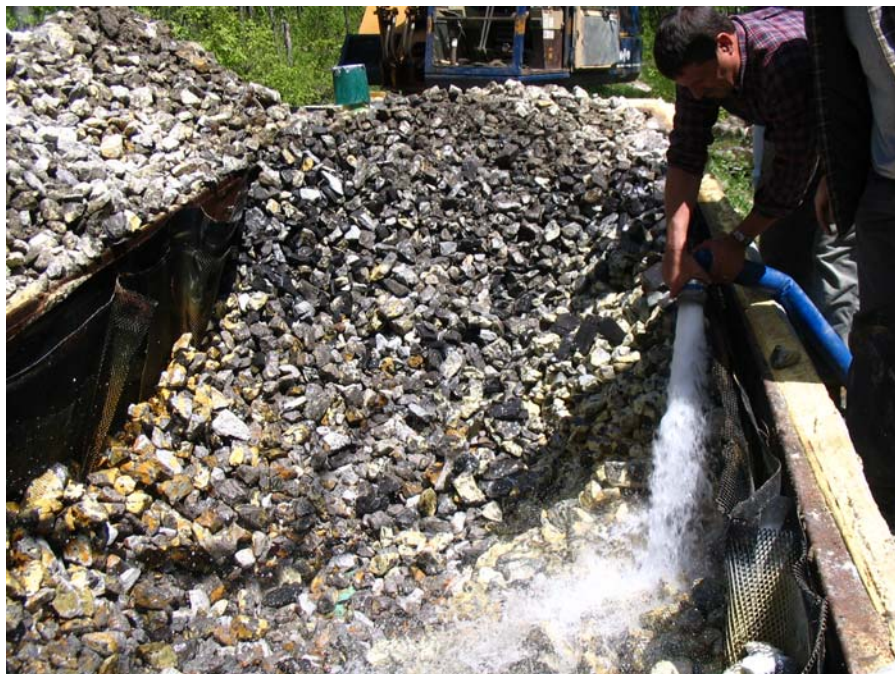
Photo 18. Washing Jon01 limestone with pumped fresh water.
