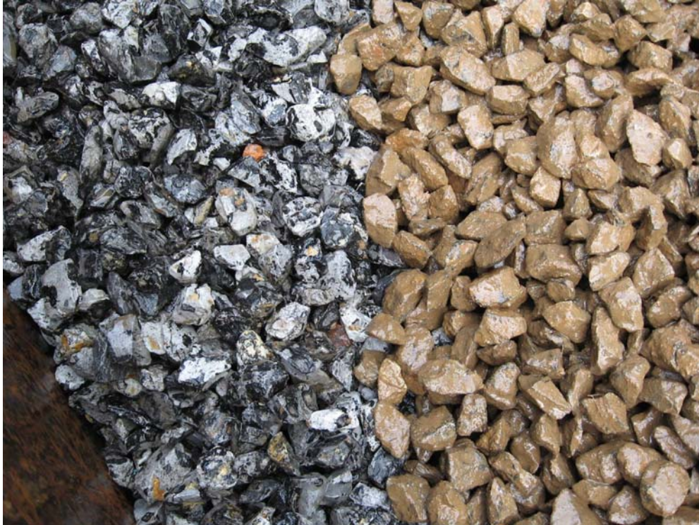
Photo 28. Comparison of cleaned limestone (left) and uncleaned limestone (right) in the East Box.
